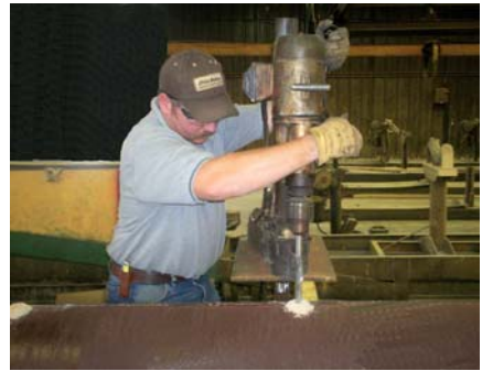
Factory hole drilling
